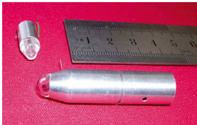
Fig. 1.1 Early, noningestible wired devices with a \frac{1}{4} -in. CCD used for testing the optics and the illumination
