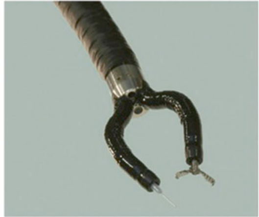
Fig. 1.3 A multi-tasking platform (EndoSAMURAI, Olympus Medical Systems). Reproduction of this image, obtained from Ikeda et al. [40], was permitted by Elsevier
